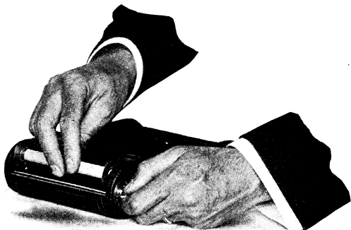
FIG. IV. Pulling out Key to admit new Reel.
